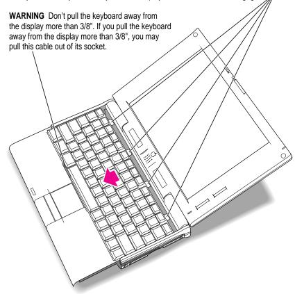
This action should move the top edge of the keyboard out of its enclosure, allowing you to grasp and free the entire keyboard.
